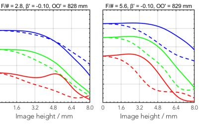
– 20 LP/mm, radial 40 LP/mm, radial 80 LP/mm, radial --- 20 LP/mm, tangential --- 40 LP/mm, tangential --- 80 LP/mm, tangential
