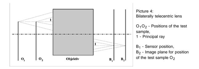
In this instance, the imaging situation corresponds to that of Diagram 2, i.e.,  $O_1$  is sharply depicted in sensor plane  $B_1$ , but from  $O_2$  a fuzzy image occurs in  $B_1$ . The significant difference in Picture 2
