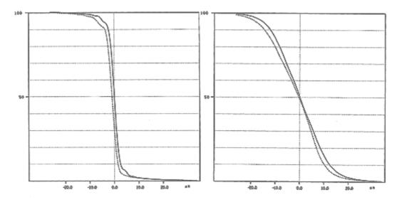
Picture 3: Edge images of a lens without image-side telecentrics exactly focused and defocused by -0.3 mm � � � radial ------ tangential
